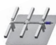
Stone Diffuser Manifold
