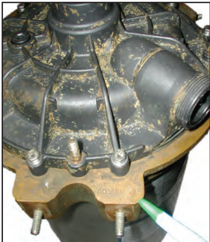
C2 Units: Engraved into brass motor ring (typically to left of bulkhead)
