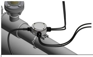
IMPORTANT FOR ALL UNITS REMOVE CABLE SLACK USING THE NYLON WIRE TIES SUPPLIED WITH EACH MR16 LED LIGHTING KIT BY FASTENING CABLES TO THE AERATOR UNIT
