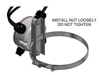
TIGHTEN BAND CLAMP WITH 7/16" NUT DRIVER (TO PREVENT DAMAGE DO NOT OVER-TIGHTEN) CONNECT POWER CABLE BEFORE LAUNCHING
