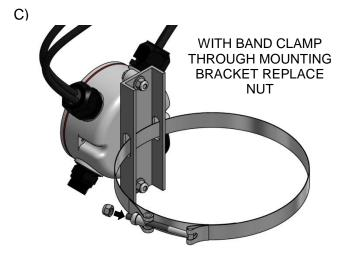
E) SLIDE J-BOX/BAND CLAMP ASSEMBLY ONTO AERATOR HOUSING
