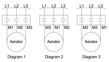
b. If the phase farthest from the average current moves on each of the connections with a particular motor lead, then the primary cause of unbalance is on the "motor side" of the circuit.
