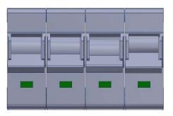
Breaker Off/Tripped (Handle Down) – 3 Phase Only Indicates a ground fault trip or circuit breaker overcurrent
