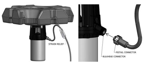
3. A small amount of silicon compound has been factory applied to the female end of the aerator connector. The compound is necessary to make a waterproof seal between the two connectors. **DO NOT REMOVE COMPOUND!** When servicing the aerator re-apply compound. (Otterbine P/N: 48-0001).
